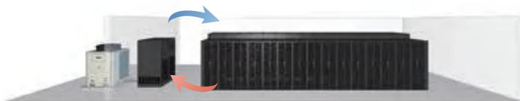
The hood guides the air to supply air, with less cooling loss, large air supply volume, good heat transfer uniformity, simple and fast construction, and is suitable for occasions with small computer rooms.
